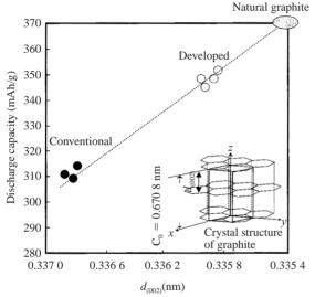
Measurement conditions of discharge capacity: Electrolyte; 1 M LiPF $_6$  in EC/EMC (1:2 volume) Discharge; Constant current to 1.5 V (1.5 V cut off) (Discharge rate: 0.1 C)
