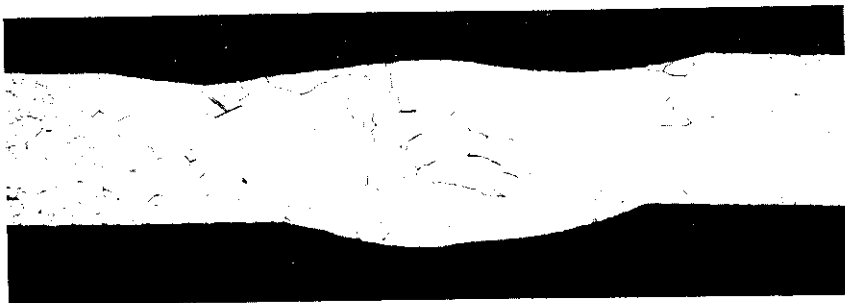
Steel A, 2mm thick, TIG 6000 J/cm
