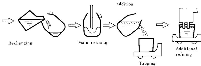
Fig. 2 An outline of the double slag refining in a LD converter
