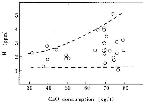
Fig. 3 Effect of CaO consumption in LD converter on hydrogen content in molten steel at blow
