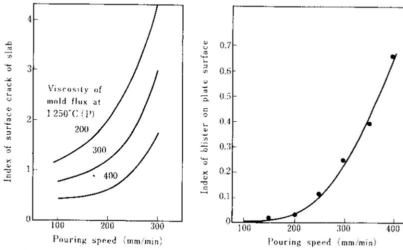
Fig. 7. Effect of bottom pouring speed on surface quality of low alloy steel.
