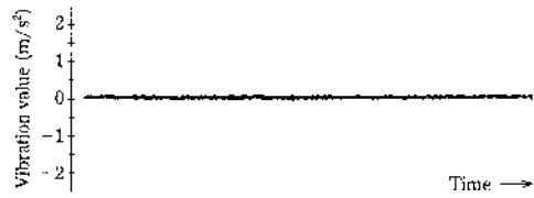
Fig. 1 Original wave form of the normal bearing
